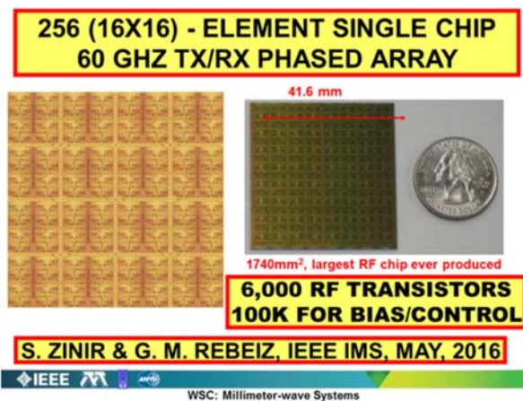
Figure 5. 256-Element 60 GHz Transmit Phased Array [9].
