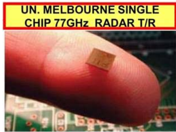
Figure 6. Un. Melbourne single chip 77 GHz Radar T/R. From G.Klari, et al, Microwave J., 1-14-15 [11].
